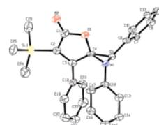
Figure 1. X-ray structure of aziridine **7a**.
